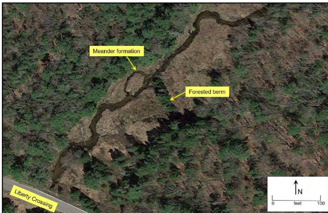
Figure 18. Google Earth image of the downstream end of Reach 17 highlighting the forested berm blocking the floodplain and the associated meander formation downstream.
